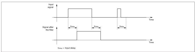
The input delay can be set in steps of 100  $\mu$ s. It makes sense, however, to enter values in steps of 2 since the input signals are sampled in an interval of 200  $\mu$ s.
