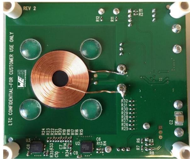
Figure 4: DC1967A, receiver demo board with WE receiver coil # 760308101303
