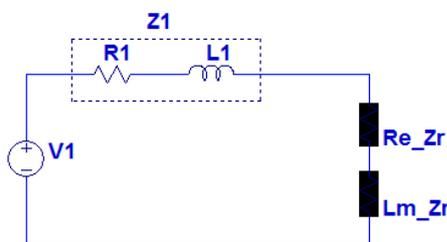
Figure 8: Equivalent primary model with reflected impedance
