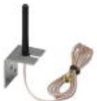
Omnidirectional antenna, 2.4 GHz, 2 dBi, linear vertical, 1.5 m cable, RSMA (male), IP65, 50 Ω impedance
