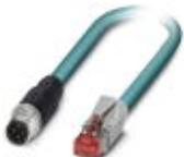
Assembled Ethernet cable, CAT5e, shielded, 2-pair, AWG 26, stranded (7-wire), RAL 5021 (aqua blue), M12 plug to RJ45 plug/IP20, line, length 1 m
