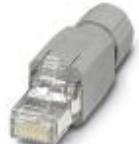
RJ45 plug-in connector, IP20, CAT5e, 8-pos., with QUICKON fast connection technology, for 26 ... 23 AWG 1-wire and 7-wire conductors, for 4.5 mm ... 8.0 mm cable diameter, labeling: TIA 568 B, color: gray
