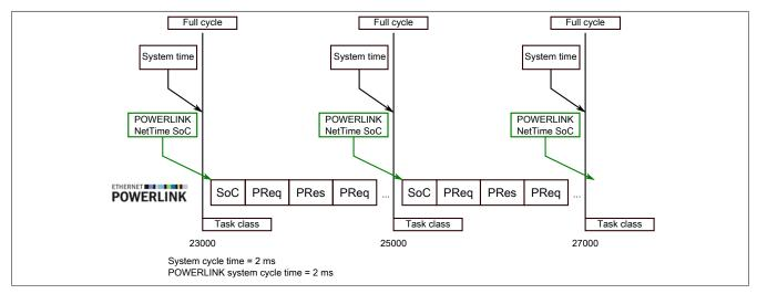
The reference moment on the POWERLINK network is always calculated at the start of cycle (SoC) of the POW-ERLINK network. The SoC starts 20 µs after the system tick. This results in the following difference between the system time and the POWERLINK reference time:
