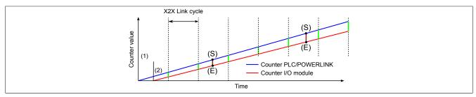
At startup, the internal counters for the PLC/POWERLINK (1) and the I/O module (2) start at different times and increase the values with microsecond resolution.
