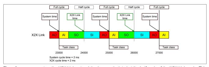
The reference moment on the X2X Link network is always calculated at the half cycle of the X2X Link cycle. This results in a difference between the system time and the X2X Link reference moment when the reference time is read out.
