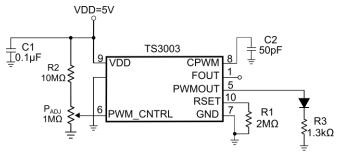
Figure 3: TS3003 Configured to Dim an LED with a Potentiometer
