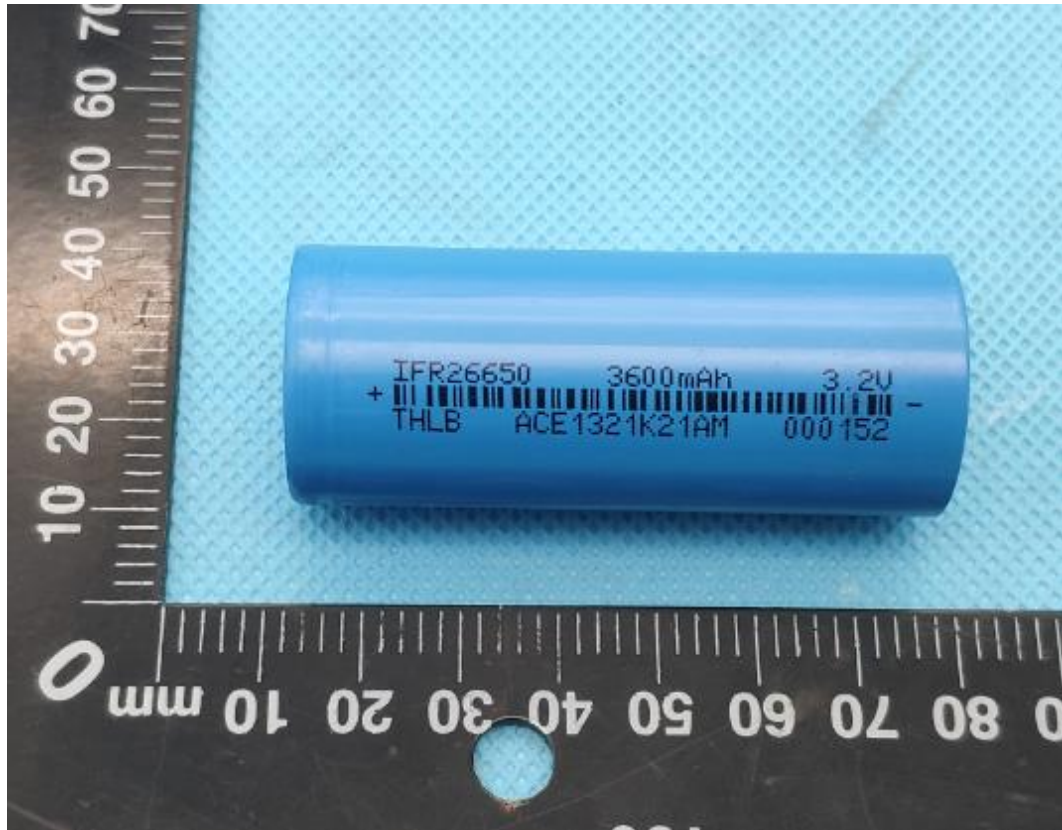
Cells /电芯 (IFR26650 3.2V 3600mAh 11.52Wh)
