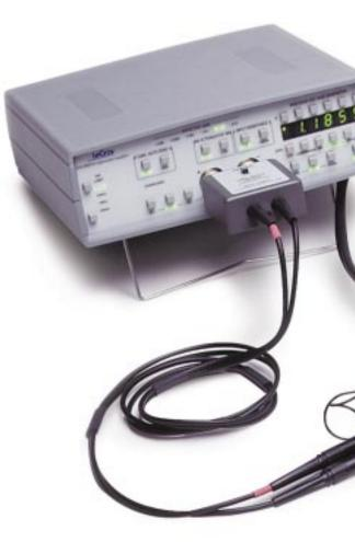
The AP015 current probe measures the current flowing through a conductor. The probe is based on a combination of Hall effect and transformer technology that allows measurements to be made on DC, AC, and impulse currents. Its rugged design uses a split-core transformer that allows the probe head to be clamped around a conductor that remains in circuit.
