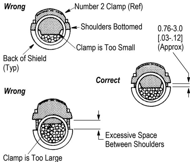
**NOTE:** These Views Represent Clamps with Fully Tightened Screws.
