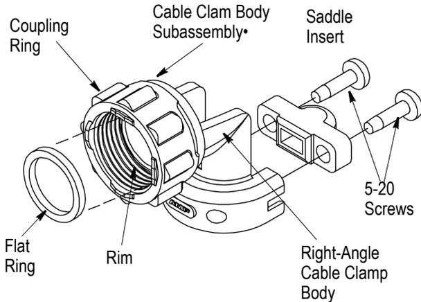
• The cable clamp body subassembly consists of the coupling ring and the right-angle cable clamp body.
