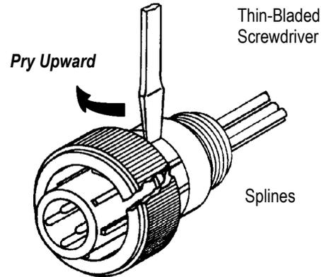
Removing Damaged Coupling Ring
