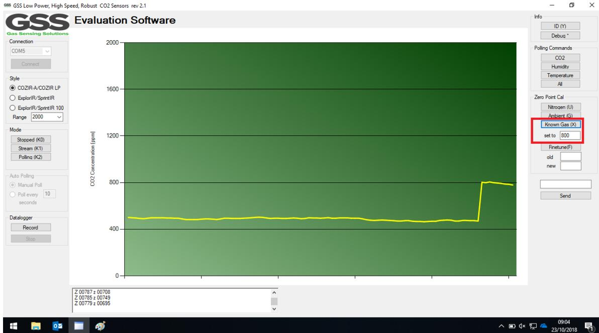
Please note, if you're using our ExplorIR® sensors you need to multiply the reading given to get the actual result. If you have a 100% concentration ExplorIR® sensor, multiply the reading by 100. For all other ExplorIR® sensors, multiply the reading by 10.
