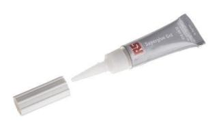
918-6885 is a medium viscosity, black rubber-toughened cyanoacrylate adhesive. The superglue displays excellent peel and impact strength and is well suited to applications involving vibration, thermal shock, temperature cycling and high humidity.
