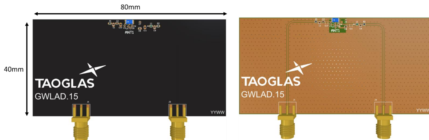
Top Side (GWLAD.15 placement on 80x40mm PCB)
