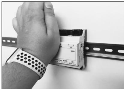
*Fig. 7: Press device onto top-hat rail*
