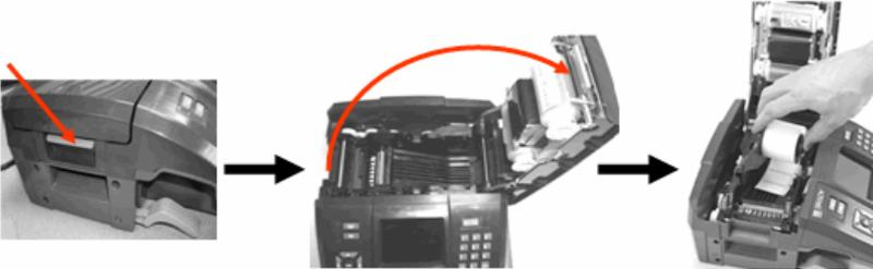
4. Insert label end up to black line under ribs.
