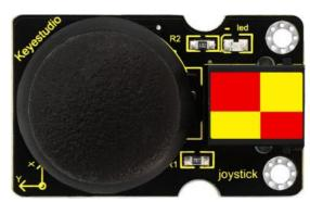
module works by reading two analog values and high/low levels at a digital port.
