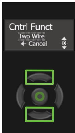
Use Up and Down arrows to set correct Control Function (Three Wire, Two Wire, DI-Prog Reset, DI-Prog Hold, DI-Prog Enable, DI-Prog Fire)
