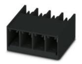
Header, nominal current: 41 A, rated voltage (III/2): 630 V, number of positions: 4, pitch: 7.62 mm, color: black, contact surface: Tin
