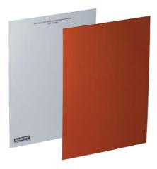
The Leica GZM26 Target Plate is a 2-sided target plate that aids in measurement of non-reflective surfaces. The grey side is intended for shorter distances and the brown sign is designed for measurement of longer distances. This item is approximately 210 x 297mm.
