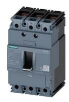
circuit breaker 3VA1 IEC frame 160 breaking capacity class N Icu=25kA @ 415V 3-pole, line protection TM210, FTFM, In=160A overload protection Ir=160A fixed short-circuit protection Ii=10 x In nut keeper kit
