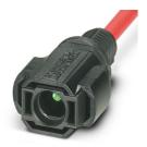
Device connector front mounting, Range of articles: SUNCLIX, color: black, number of positions: 1, min. conductor cross section: 6 mm², Connection method: Crimp, Contact connection type: Pin, cable length: 300
