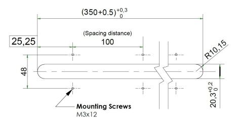
If IP65 is not needed, the amount of **Clip** can be Reduced. And **Spacing distance** can user-defined.
