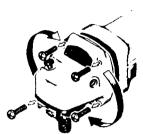
The machine head can be turned on the motor housing in 90 degree steps. In this manner, the on-off switch can be brought into a favourable handling position for special working situations, e. g., for cutting work with the cutting guide/cutting stand 18 (accessories) and also for left handed persons.
