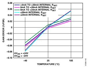
Figure 43. Gain Error vs. Temperature, Internal R<sub>SET</sub> Sense Resistor
