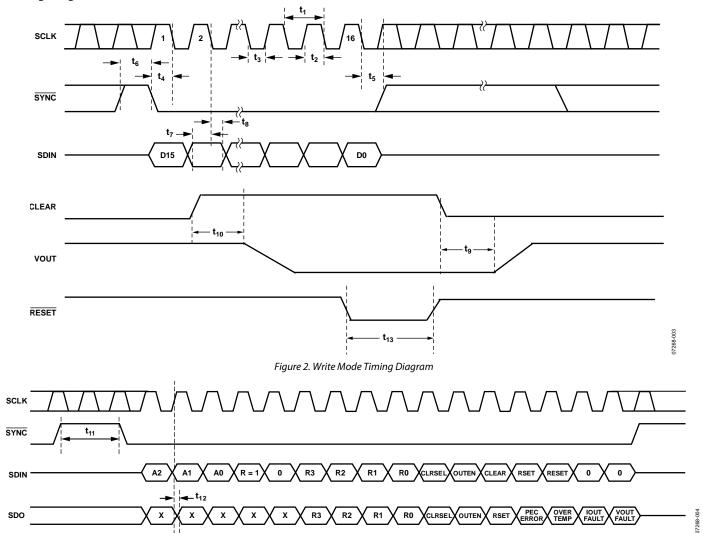
Figure 3. Readback Mode Timing Diagram
