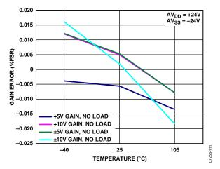
Figure 11. Gain Error vs. Temperature
