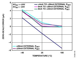
Figure 36. Zero-Scale Error vs. Temperature, External R<sub>SET</sub> Sense Resistor
