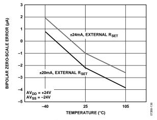
Figure 38. Bipolar Zero-Scale Error vs. Temperature, External R<sub>SET</sub> Sense Resistor
