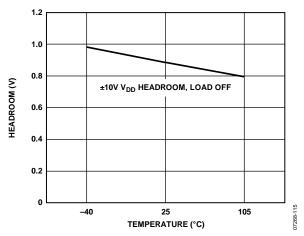
Figure 15. AV<sub>DD</sub> Headroom, ±10 V Range, Output Set to 10 V, Load Off
