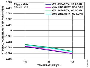
Figure 6. Integral Nonlinearity Error vs. Temperature
