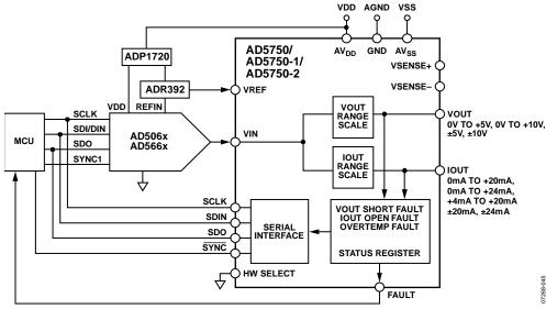
Figure 51. Typical System Configuration in Software Mode (Pull-Up Resistors Not Shown for Open-Drain Outputs)
