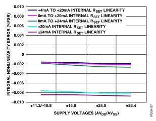
Figure 27. Integral Nonlinearity Error, Current Mode, Internal R<sub>SET</sub> Sense Resistor
