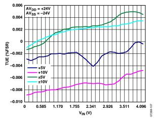
Figure 7. Total Unadjusted Error (TUE) vs. V<sub>IN</sub>
