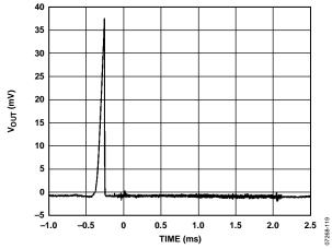
Figure 19.  $V_{OUT}$  vs. Time on Power-Up, Load =  $2 k\Omega \parallel 200 pF$
