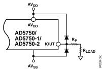
Figure 56. Output Transient Voltage Protection
