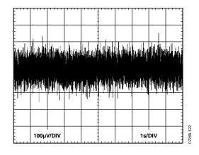
Figure 22. Peak-to-Peak Noise (100 kHz Bandwidth)
