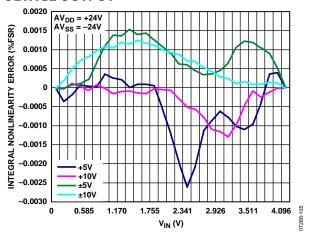
Figure 5. Integral Nonlinearity Error vs.  $V_{IN}$
