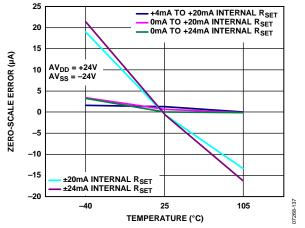
Figure 37. Zero-Scale Error vs. Temperature, Internal R<sub>SET</sub> Sense Resistor
