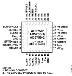
Figure 4. Pin Configuration
