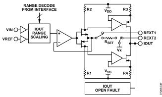
Figure 53. Current Output Configuration
