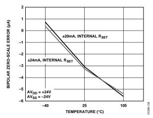
Figure 39. Bipolar Zero-Scale Error vs. Temperature, Internal R<sub>SET</sub> Sense Resistor
