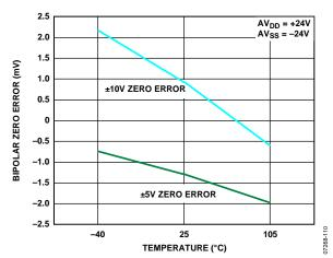
Figure 10. Bipolar Zero Error vs. Temperature
