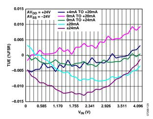
Figure 29. Total Unadjusted Error vs. V<sub>IN</sub>, Internal R<sub>SET</sub> Resistor
