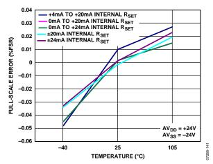
Figure 41. Full-Scale Error vs. Temperature, Internal R<sub>SET</sub> Sense Resistor
