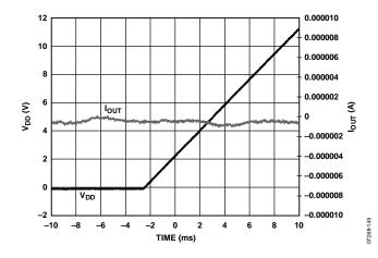
Figure 45. V<sub>DD</sub> and Output Current (I<sub>OUT</sub>) vs. Time-On Power-Up
