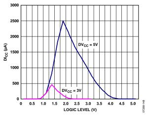
Figure 48. Dlcc vs. Logic Input Voltage
