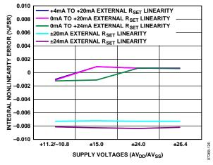
Figure 26. Integral Nonlinearity Error, Current Mode, External R<sub>SET</sub> Sense Resistor
