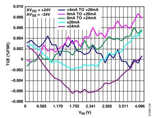
Figure 28. Total Unadjusted Error (TUE) vs. V<sub>IN</sub>, External R<sub>SET</sub> Resistor
