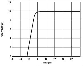
Figure 17. Full-Scale Positive Step
