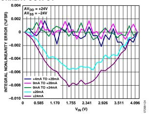
Figure 24. Integral Nonlinearity Error vs. V<sub>IN</sub>, External R<sub>SET</sub> Resistor
