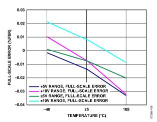
Figure 9. Full-Scale Error vs. Temperature
