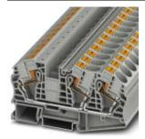
Feed-through terminal block, Connection method: Push-in connection, Cross section: 0.5 mm<sup>2</sup> - 25 mm<sup>2</sup>, AWG: 20 - 4, Width: 12.2 mm, Color: gray, Mounting type: NS 35/7,5, NS 35/15
