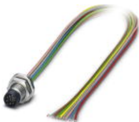
Sensor/actuator flush-type plug, 8-pos., M8, rear/screw mounting with M8 fastening thread, with 0.5 m TPE litz wire, 8 x 0.14 mm 2
