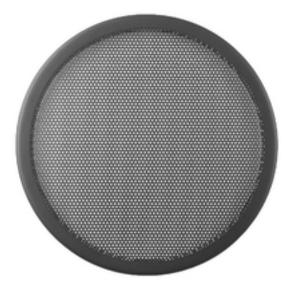
Decorative Speaker Grilles With fine perforation, 2-part version with fixing ring to be screwed for the speaker and push-on grille, various sizes. Decorative speaker grilles, two parts, for the most common standard speaker sizes. Mounting rim serves for mounting the speaker; cover rim with metal grille covers speaker and mounting completely.
