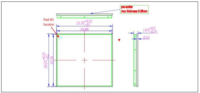
Figure 4. Module Top and Side View and Dimensions
