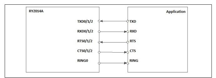
Figure 10. UART0, UART1 and UART2 Signals Convention and Flow Control
