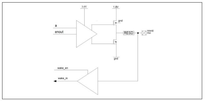
Figure 14. PMU Wake IOs in Sleep Mode or Active Mode
