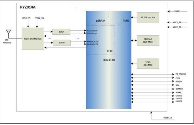
Figure 1. RYZ014A Block Diagram
