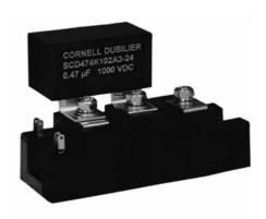
Style SCD offers protection against voltage transients in low to medium current IGBT applications where high dV/dt is encountered. Connect these capacitors from C1 to E2 on a dual IGBT module or from P to N on a six-pack module to eliminate severe voltage transients. Parts ending with Z25 fit IGBTs with 23mm, 25mm and 28mm lead spacing. If you have a preferred lead spacing, please specify.
