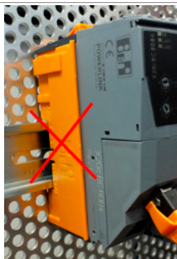
Figure 3: X20 system - Removing the end cover plates
