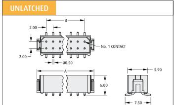
Friction lock or latch (when fitted) adds 0.5mm to overall length 'A'
