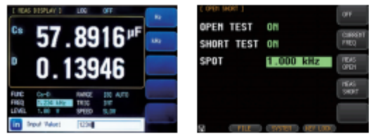
Consecutive and Adjustable Frequency Freely Input Frequency Within Provided Frequency Range Selectable Fixture Zeroing Methods Full Frequency Range Zero or Spot Zero
