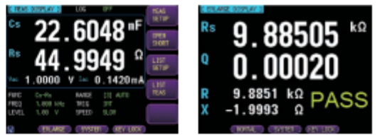
MEAS Display Parameter Setting and Four Measurement Parameters ENLARGE Display Enlarge Measurement Results and Include PASS/FAIL Judgment
