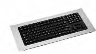
Plate is 14 gauge steel finished with RAL 7035 light-gray textured polyester powder paint or Type 304 stainless steel with a brushed finish. Available blank or with TIP NEMA 4 Keyboard. Includes mounting hardware.
