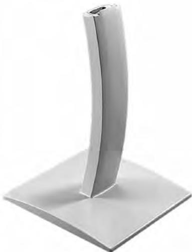
Pedestal can be bolted to the floor or mounted on accessory swivel casters. Center channel is 2 x 3 in. with rear access strip for routing wires. Requires single or dual tilt for enclosure mounting. Finished with RAL 7035 light-gray polyester powder paint.
