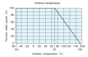
For resistors operated at an ambient temperature of  $70{^\circ}\!{\rm C}$  or higher, the power shall be derated in accordance with the above derating curve.
