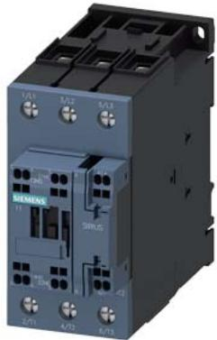
traction contactor, AC-3e/AC-3, 51 A, 22 kW / 400 V, 3-pole, 110 V DC, 0.7-1.25\* Uc, solid-state operating mechanism, with integrated varistor, auxiliary contacts: 1 NO + 1 NC, main circuit: screw terminal, control and auxiliary circuit: spring-loaded terminal, frame size: S2
