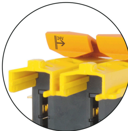
Figure 3: X20BM2x - Voltage routing identification
