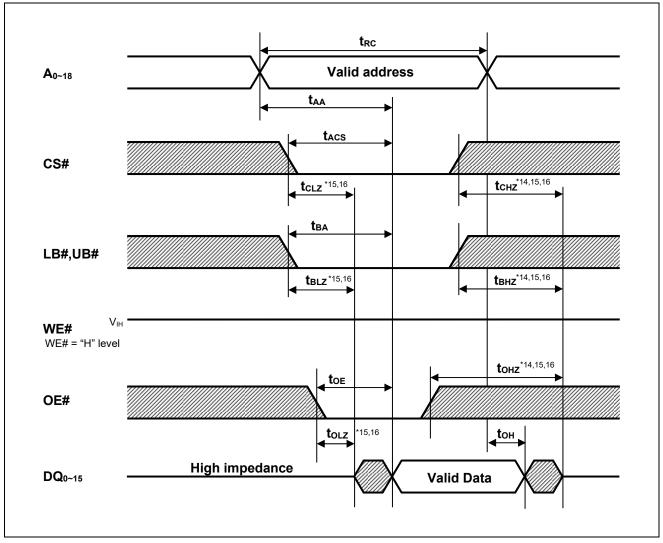
Note 14.  $t_{CHZ}$ ,  $t_{BHZ}$  and  $t_{OHZ}$  are defined as the time when the DQ pins enter a high-impedance state and are not referred to the DQ levels.
