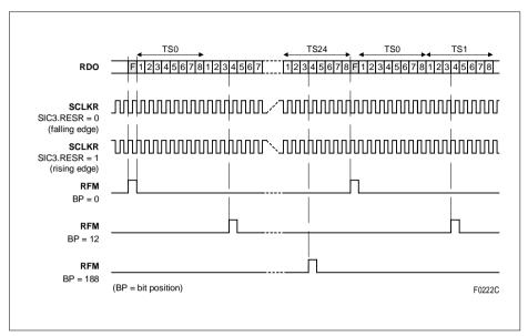
Figure 58 RFM Offset Programming (1.544 Mbit/s, 1.544 MHz)
