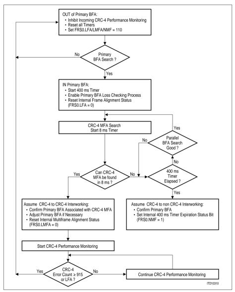
Figure 22 CRC4 Multiframe Alignment Recovery Algorithms (E1)
