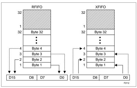
Figure 8 FIFO Word Access (Intel Mode)
