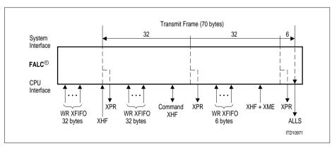
Figure 79 Interrupt Driven Transmission Example
