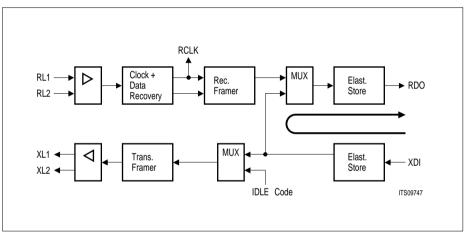
Figure 75 Channel Loop-Back (T1/J1)
