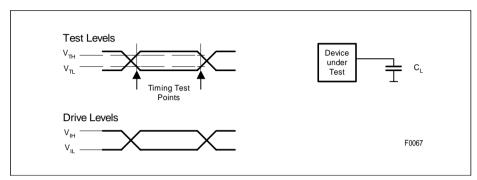
Figure 106 Input/Output Waveforms for AC Testing
