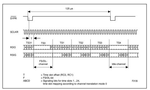
Figure 60 2.048 MHz Receive Signaling Highway (T1/J1)
