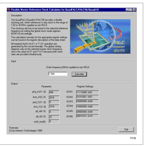
Figure 109 Master Clock Frequency Calculator
