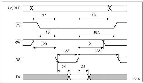
Figure 88 Motorola Read Cycle Timing
