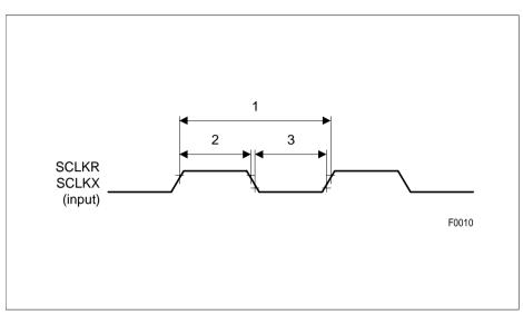
Figure 93 SCLKR/SCLKX Input Timing
