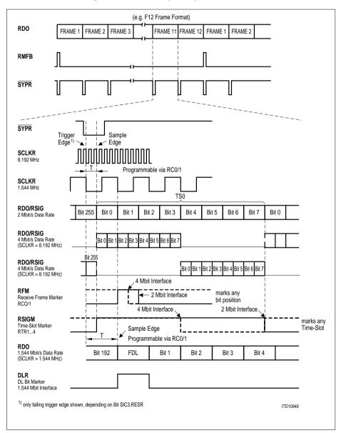
Figure 55 Receive System Interface Clocking (T1/J1)
