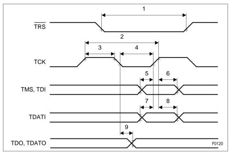
Figure 82 JTAG Boundary Scan Timing
