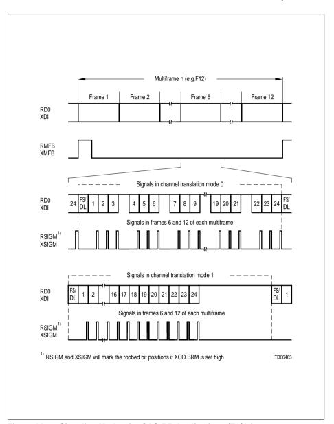
Figure 68 Signaling Marker for CAS-BR Applications (T1/J1)
