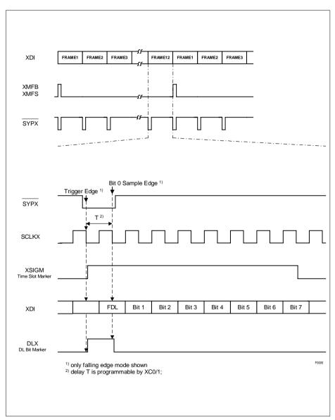
Figure 63 Transmit System Clocking: 1.544 MHz (T1/J1)
