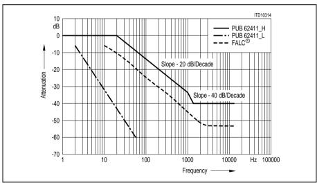
Figure 45 Jitter Attenuation Performance (T1/J1)
