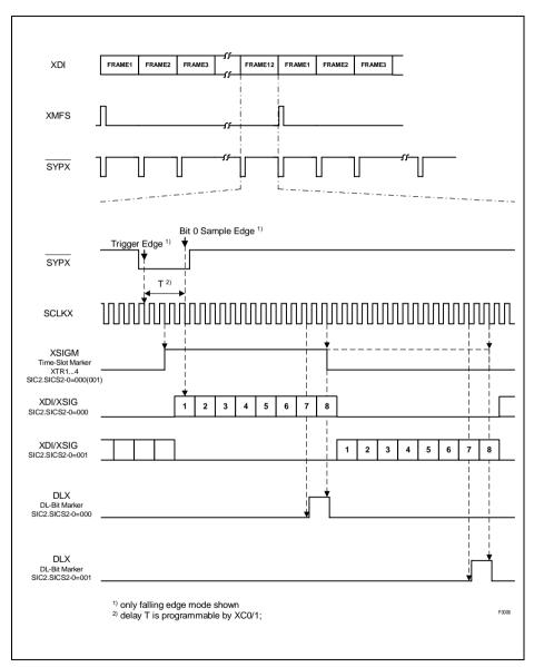
Figure 64 Transmit System Clocking: 8.192 MHz/4.096 Mbit/s (T1/J1)
