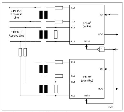
Figure 44 Protection Switching Application
