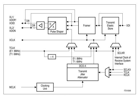
Figure 24 Transmit Clock System (E1)
