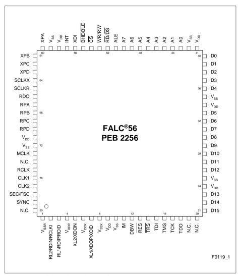
Figure 4 Pin Configuration P-MQFP-80-1
