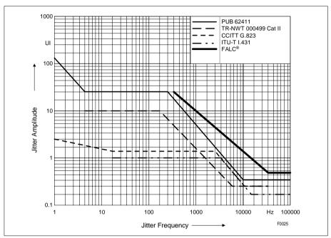
Figure 18 Jitter Tolerance (E1)
