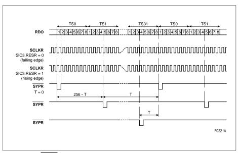
Figure 29 SYPR Offset Programming (2.048 Mbit/s, 2.048 MHz)
