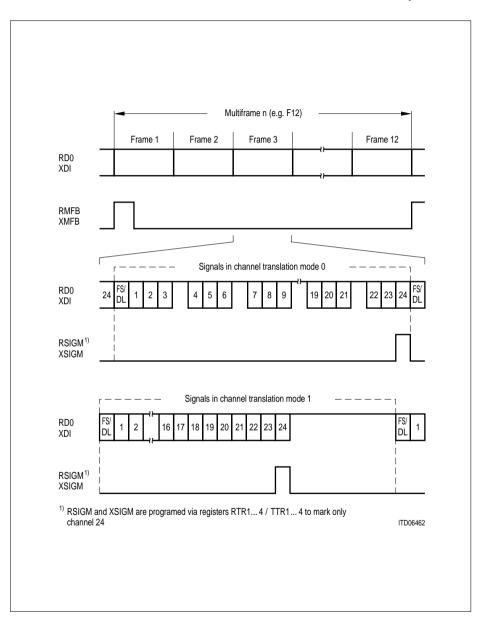
Figure 67 Signaling Marker for CAS/CAS-CC Applications (T1/J1)
