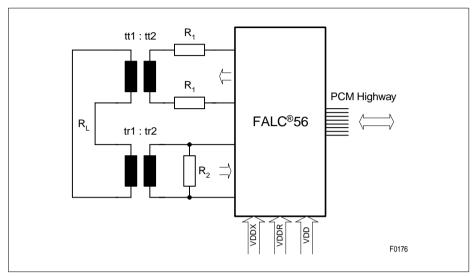
Figure 107 Device Configuration for Power Supply Testing
