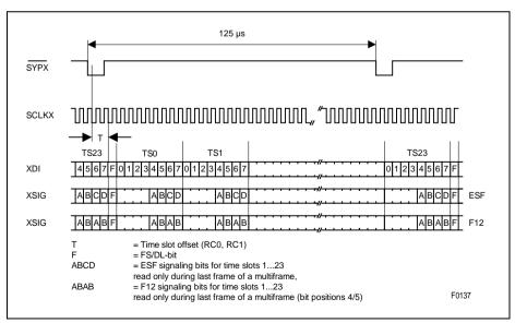
Figure 66 1.544 MHz Transmit Signaling Highway (T1/J1)
