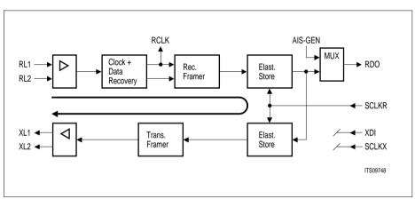
Figure 38 Payload Loop (E1)
