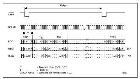
Figure 62 1.544 MHz Receive Signaling Highway (T1/J1)
