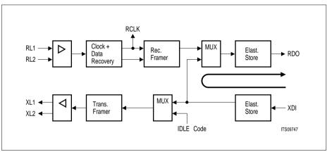
Figure 40 Single Channel Loop-Back (E1)
