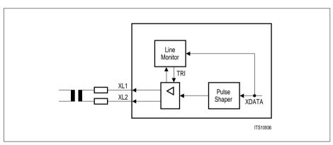
Figure 53 Transmit Line Monitor Configuration (T1/J1)
