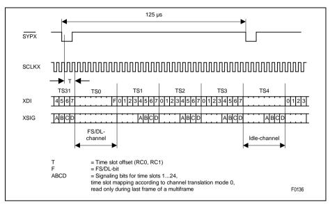
Figure 65 2.048 MHz Transmit Signaling Clocking (T1/J1)
