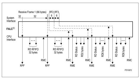
Figure 80 Interrupt Driven Reception Sequence Example
