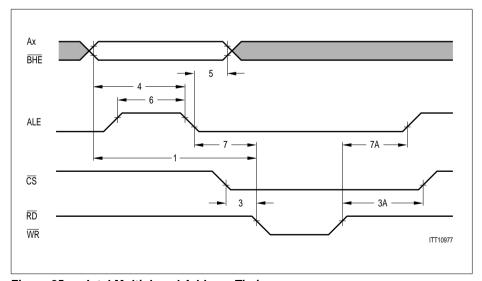
Figure 85 Intel Multiplexed Address Timing
