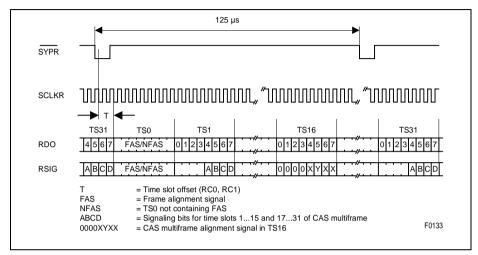
Figure 21 2.048 MHz Receive Signaling Highway (E1)
