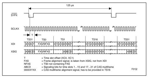
Figure 26 2.048 MHz Transmit Signaling Highway (E1)
