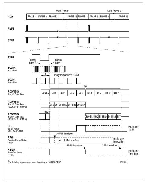
Figure 28 Receive System Interface Clocking (E1)
