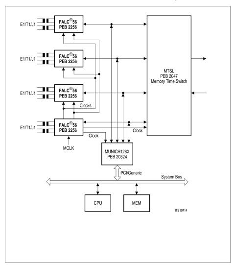
Figure 2 Multiple E1/T1/J1 Link over Frame Relay
