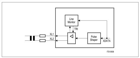
Figure 25 Transmit Line Monitor Configuration (E1)
