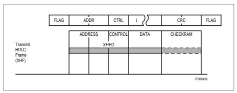
Figure 77 HDLC Transmit Data Flow
