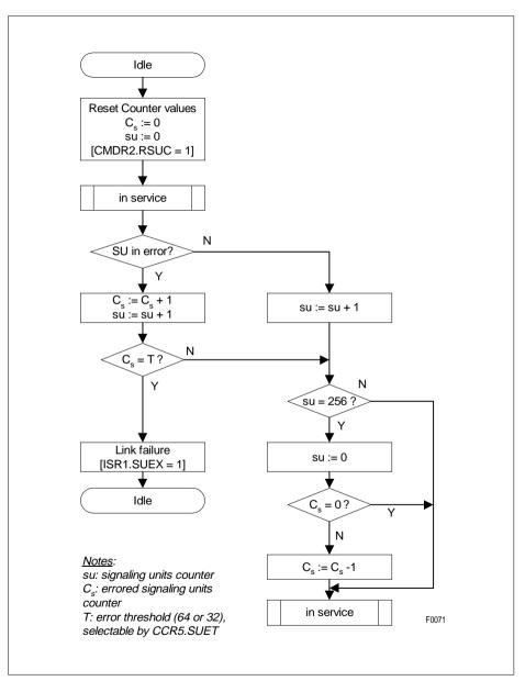
Figure 48 Automatic Handling of Errored Signaling Units
