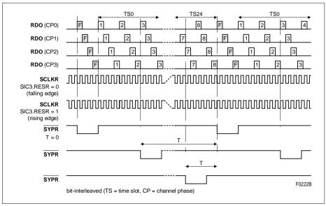
Figure 57 SYPR Offset Programming (6.176 Mbit/s, 6.176 MHz)
