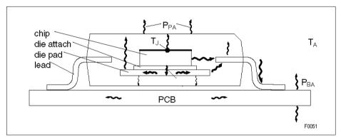
Figure 105 Thermal Behavior of Package
