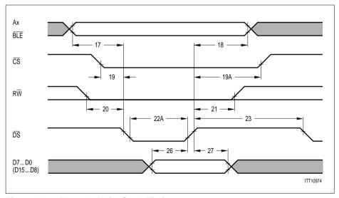
Figure 89 Motorola Write Cycle Timing
