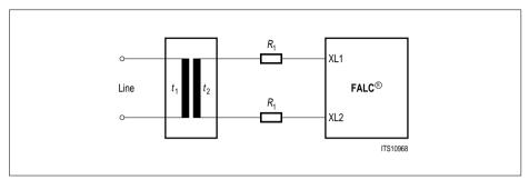
Figure 50 Transmitter Configuration (T1/J1)
