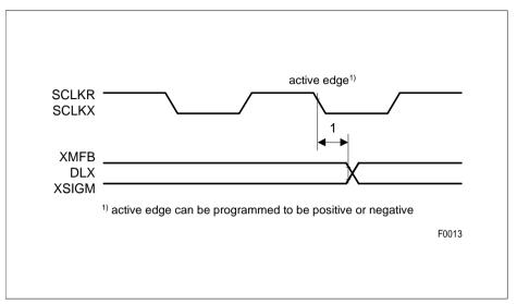
Figure 96 System Interface Marker Timing (Transmit)
