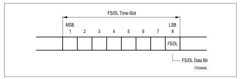
Figure 69 Transmit FS/DL Bits on XDI (T1/J1)
