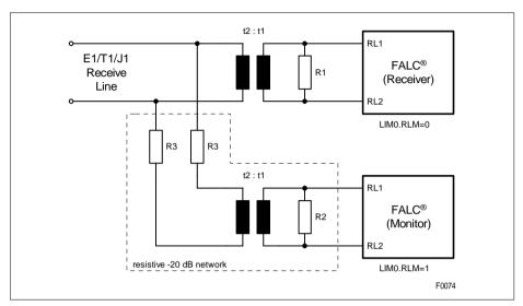
Figure 15 Receive Line Monitoring
