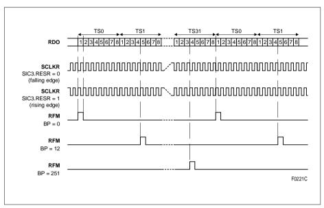
Figure 31 RFM Offset Programming (2.048 Mbit/s, 2.048 MHz)
