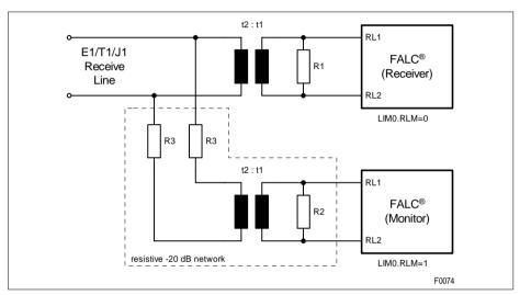
Figure 43 Receive Line Monitoring
