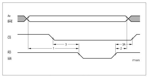
Figure 84 Intel Non-Multiplexed Address Timing
