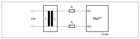
Figure 23 Transmitter Configuration (E1)
