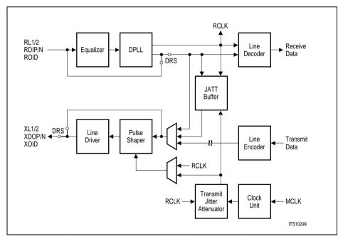
Figure 51 Clocking in Remote Loop Configuration (T1/J1)
