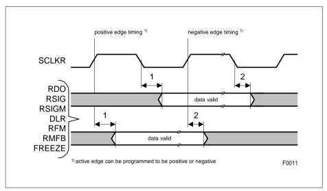
Figure 94 System Interface Marker Timing (Receive)
