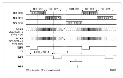
Figure 30 SYPR Offset Programming (8.192 Mbit/s, 8.192 MHz)
