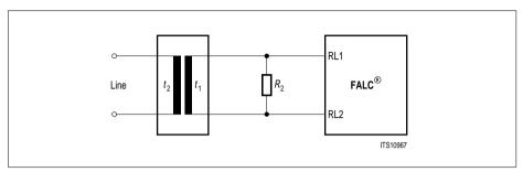
Figure 42 Receiver Configuration (T1/J1)
