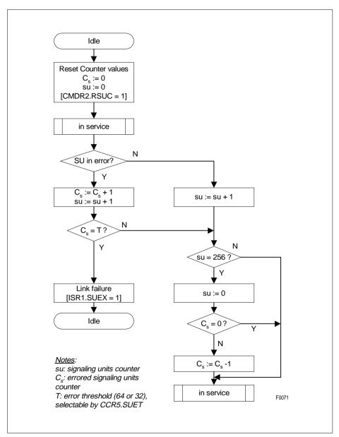
Figure 20 Automatic Handling of Errored Signaling Units
