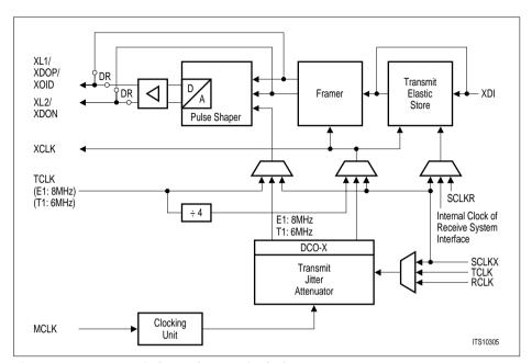
Figure 52 Transmit Clock System (T1/J1)
