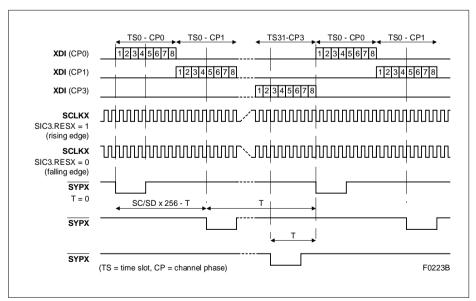
Figure 36 SYPX Offset Programming (8.192 Mbit/s, 8.192 MHz)
