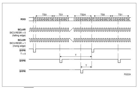
Figure 56 SYPR Offset Programming (1.544 Mbit/s, 1.544 MHz)
