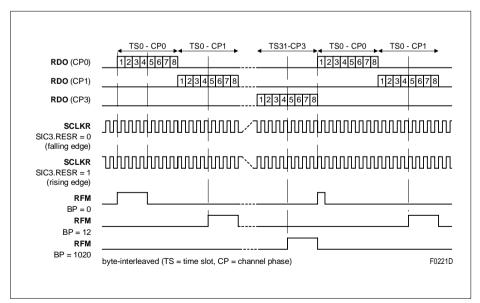
Figure 32 RFM Offset Programming (8.192 Mbit/s, 8.192 MHz)
