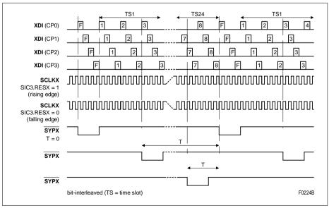
Figure 71 SYPX Offset Programming (6.176 Mbit/s, 6.176 MHz)
