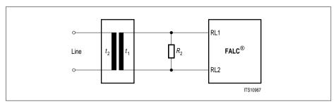
Figure 14 Receiver Configuration (E1)
