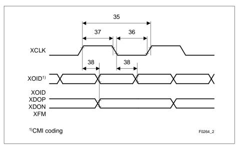
Figure 91 Digital Line Interface Transmit Timing
