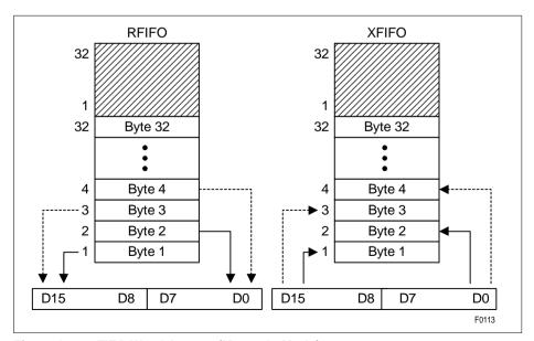
Figure 9 FIFO Word Access (Motorola Mode)
