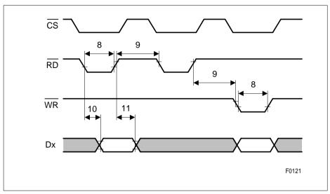
Figure 86 Intel Read Cycle Timing
