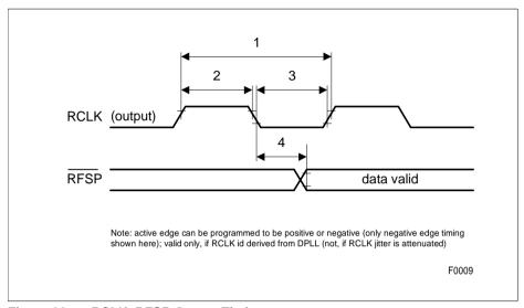
Figure 92 RCLK, RFSP Output Timing
