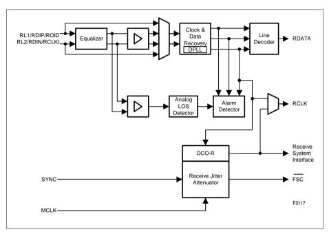
Figure 13 Receive Clock System (E1)
