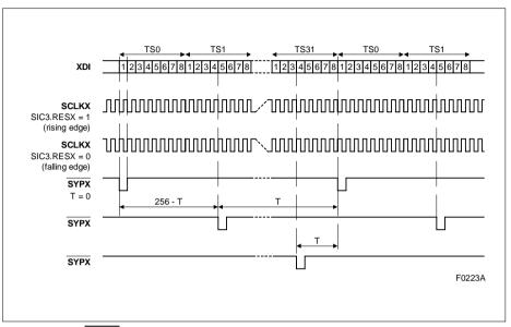
Figure 35 SYPX Offset Programming (2.048 Mbit/s, 2.048 MHz)
