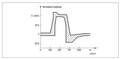
Figure 104 T1 Pulse Shape at the Cross Connect Point
