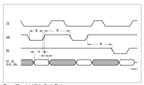
Figure 87 Intel Write Cycle Timing
