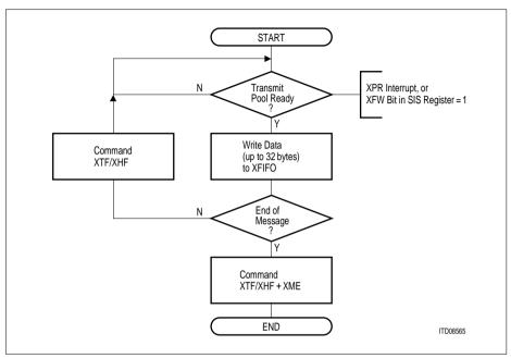
Figure 78 Interrupt Driven Data Transmission (flow diagram)
