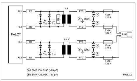
Figure 108 Protection Circuitry Examples
