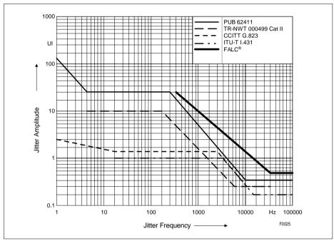
Figure 46 Jitter Tolerance (T1/J1)
