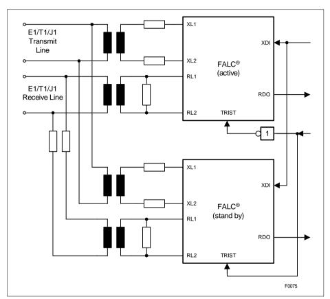
Figure 16 Protection Switching Application
