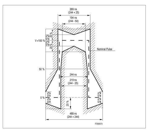
Figure 103 E1 Pulse Shape at Transmitter Output
