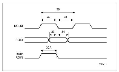
Figure 90 Digital Line Interface Receive Timing
