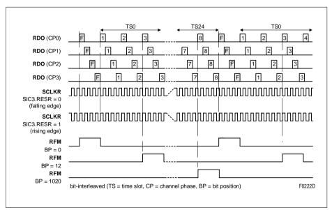
Figure 59 RFM Offset Programming (6.176 Mbit/s, 6.176 MHz)
