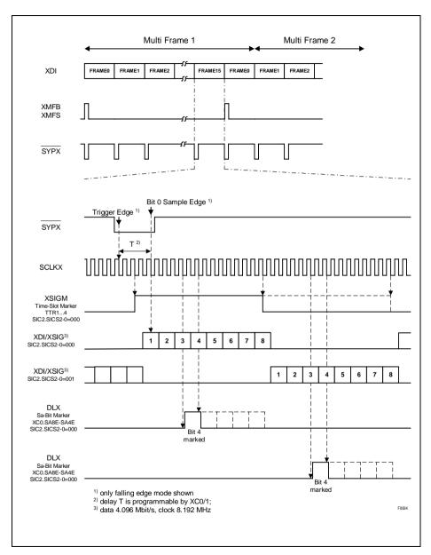
Figure 34 Transmit System Interface Clocking: 8.192 MHz/4.096 Mbit/s (E1)
