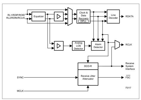
Figure 41 Receive Clock System (T1/J1)
