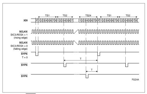
Figure 70 SYPX Offset Programming (1.544 Mbit/s, 1.544 MHz)
