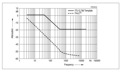
Figure 17 Jitter Attenuation Performance (E1)
