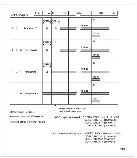
Figure 76 HDLC Receive Data Flow
