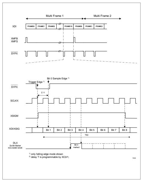
Figure 33 Transmit System Interface Clocking: 2.048 MHz (E1)
