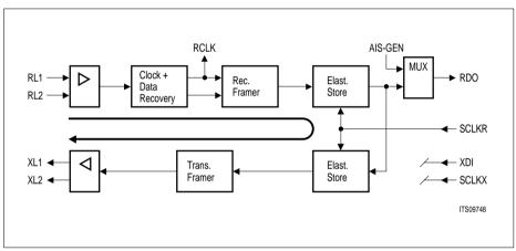
Figure 73 Payload Loop (T1/J1)
