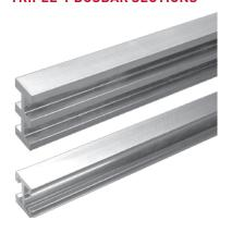
Use in higher-current applications between 756 A and 2,000 A (please contact Hoffman regarding how to achieve 4,000 A). The outer-most section of these symmetrical profile busbars are 30 x 10 mm. All 60-mm system components can be mounted on systems using this busbar structure.
