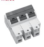
DIN Rail mountable fuse holders for 30 and 60 A ferrule size UL Class J fuses. Offered in single pole, 2-pole or 3-pole configurations with LED open fuse indication. Indicator operates on systems between 110 and 600 V. The LED lamp will glow when the fuse is open (blown). Holders meet IP20 touchsafe design standards. AMBUS J-Carrier is a trademark of Wöhner GmbH & Co. KG.
