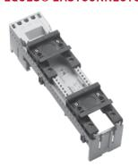
DIN rail adapters for components that have a 35-mm symmetrical DIN rail mounting provision. Available in 45-mm or 54-mm widths and 200-mm or 260-mm heights with one or two DIN rails. Most commonly used to add width to a powered EQUES EasyConnector for reversing contactor applications or to mount other components that are wider than 81 mm. The side-mounted module adds width to any adapter in 9-mm increments and maintains the IP20 fingersafe design of the busbar system.
