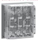
Blade size Class J bus-mounting fuse holders in 100 A, 200 A and 400 A frame sizes. Connection on bottom or top, 3-pole, 30 x 10, Double-T and Triple-T busbar sections. QUADRON J-Carrier is a trademark of Wöhner GmbH & Co. KG.
