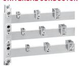
Terminals for round American Wire Gauge (AWG) conductor are used to either supply power to or draw power from the busbar system. These parts must match the thickness of the busbar being applied in your system. Cover caps are sold separately. Sold in sets of three terminals.
