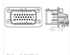
TE Part #1-776087-2 23POS,PIN DIA 1.3,HDR ASSY,90DEG, COD 2
