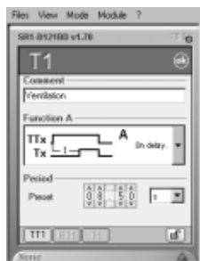
Configuration of a time delay function block
