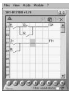
Inputting of a control scheme
