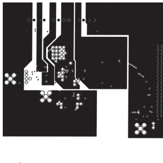
Figure 16. PCB Power Layers—Layers 3 and 4
