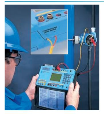
Direct connection of thermocouple compensation wires eliminates the need for special connectors and reduces additional cold junction errors. This is the most reliable and accurate method of monitoring cold junction temperatures in a portable field calibrator.
