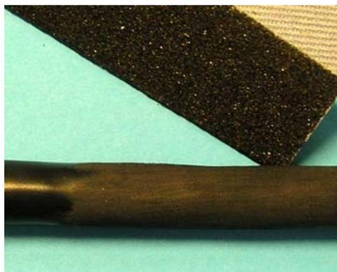
**This part of the cable preparation is very important in ensuring a strong bond to the moulded part.**
