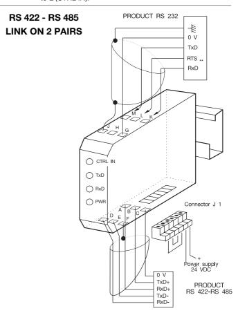
\*\* NOTE: Only to be connected for RS 485 two pairs (of no use for RS 422 two pairs). If the RTS signal is not generated, connect M (RxD ILPH) to L (CTRL IN).
