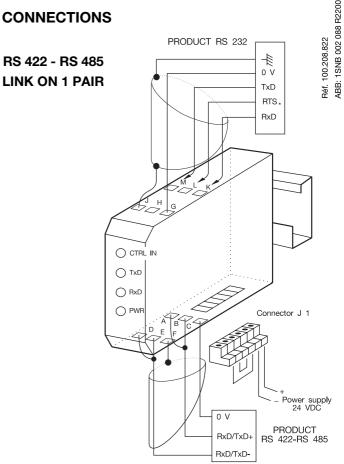
\* NOTE: If the RTS signal is not generated, connect M (RxD ILPH) to L (CTRL IN).
