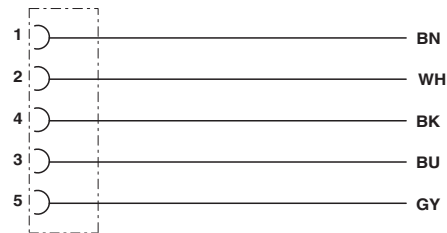
Contact assignment of the M12 sockets
