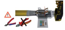
6. Lock the wire manager to the RJ45 connector body with an audible "click".
