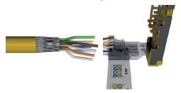
5. Insert single wires into the wire manager according to the selected terminal assignment. Assemble the lower wires first, followed by the upper wires. Cut the 4 upper wires with small cutting pliers close to the flange of the wire manager.
