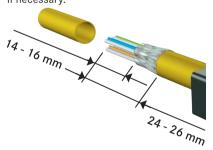
To ensure an easy RJ Industrial 10G assembly, please check the wire stripping length with the help of the scale shown below.
