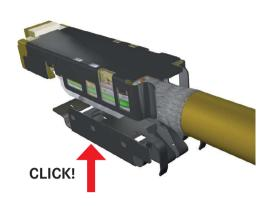
8. Push the housing over the installed data module. Use the RJ45 adapter if necessary. Fix the adapter with the screw or snap it onto the insert with an audible "click". Please use alignment symbols, if applicable, to push the hood over the insert until it snaps into place. Tighten the cable screw.
