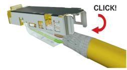
7. Lock the shield to the RJ45 plug with an audible "click".
