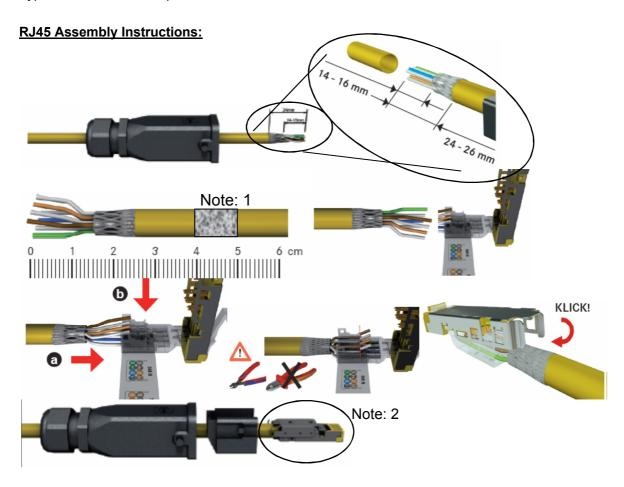
**Note#1:** To create the shield to the backshell, the cable outer sheath shall be stripped local to the cable gland.
