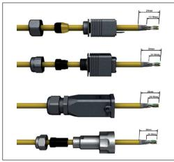
Strip the cable jacket in the length of 24-26 mm and push the cable shielding 14-16 mm back or cut it off if necessary.
