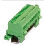
Plug component, Nominal current: 8 A, Rated voltage (III/2): 160 V, Number of positions: 16, Pitch: 3.81 mm, Connection method: Screw connection with tension sleeve, Color: green, Contact surface: Tin, Mounting: DIN rail
