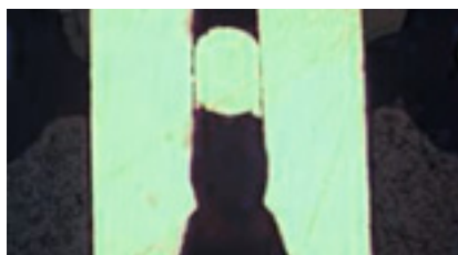
Cross Section ribbon cable AWG-26 solid wire 90° cable outlet
