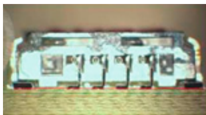
Cross Section Right Angle Male Connector
