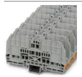
Bolt connection terminal block, Connection method: Bolt connection, Number of positions: 1, Cross section: 6 mm² - 70 mm², AWG: 8 - 2/0, Width: 29 mm, Height: 66 mm, Color: black/yellow, Mounting type: NS 35/7,5, NS 35/15, ct screw connection
