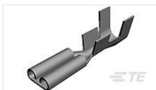
TE Part #170213-2 250 FASTON,REC.,18-14 AWG,TPBR
