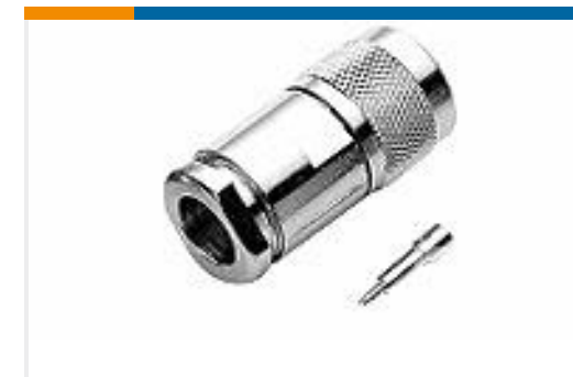
TE Part #1-1478420-0 N Str Plg PS 50Ohm Silver Pltd PSF1/4M,
